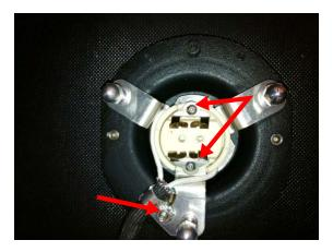
7. Install lamp cap into unit without lamp installed.
