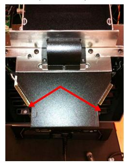
**3.** Use a flat head screwdriver to disconnect lamp wires in terminal block. Remove ground wire using 7mm nut driver.
