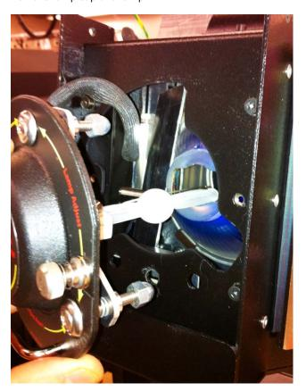
**6.** Replace lamp harness socket assembly using 2mm hex and 7mm nut driver.
