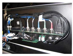
New cable routing above PCB
